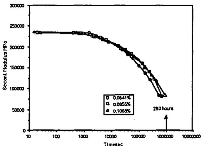
Figure 15 Secant modulus for #4 at 1350C
