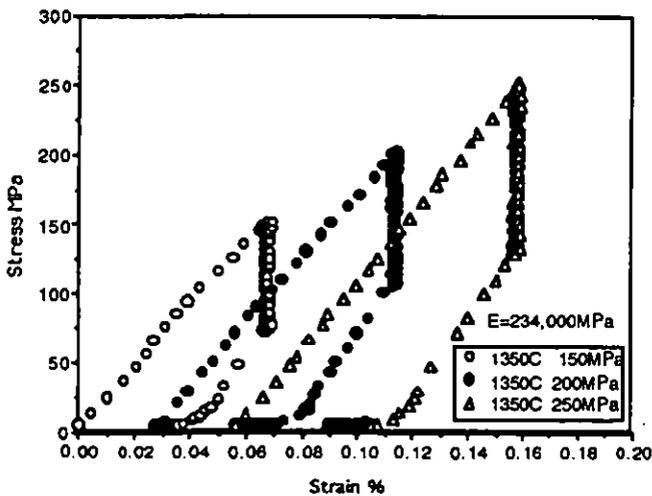
Figure 2 Stress-strain for specimen #4 at 1350C
