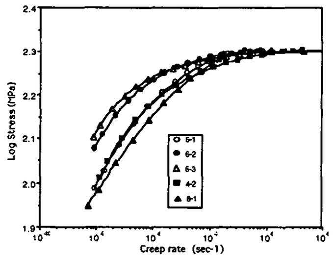
Figure 7 Specimens 6, 4 and 8 relaxed from 200MPa and 1350C
