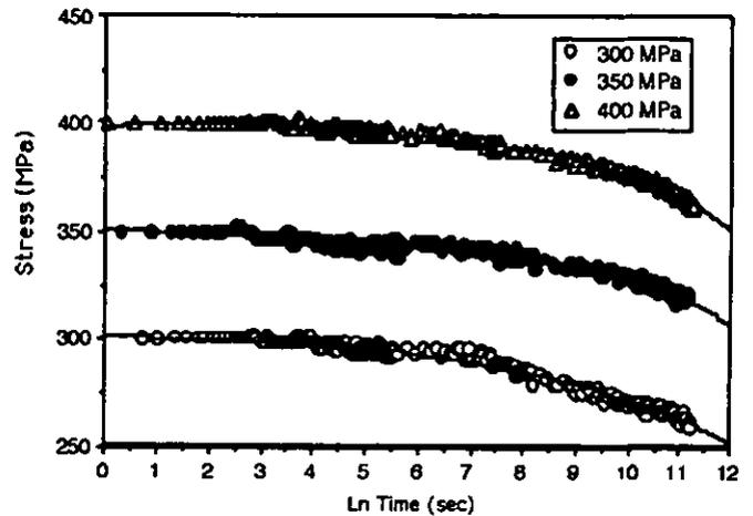
Figure 3 Stress relaxation in specimen #1 at 1200C
