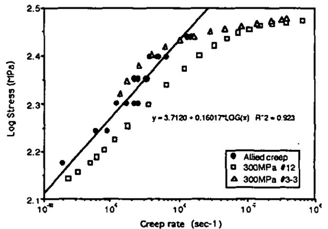
Figure 12 Comparison with Creep data at 1300C
