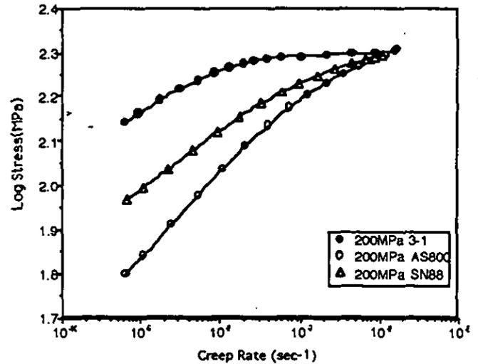
Figure 11 Comparison Data at 1300C from 200MPa
