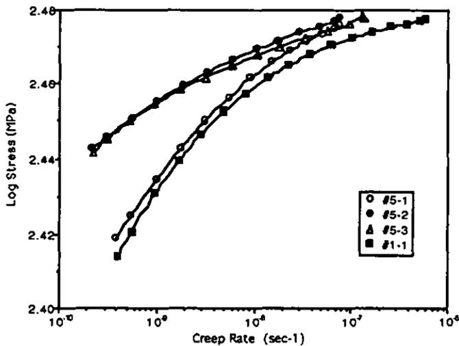
Figure 6 Specimens 5 and 1 relaxed from 300MPa and 1200C
