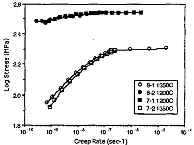
Figure 8 Effect of test sequence in specimens 7 and 8
